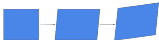
Fig. 7. Affine warping in two shears [32].
