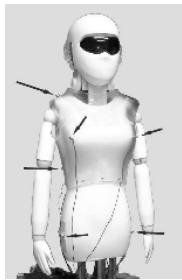
Fig. 6 SIG2 with eight microphones
