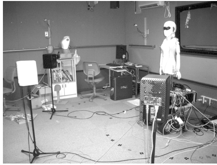
Fig. 7 SIG2 and three loudspeakers in experiment room
